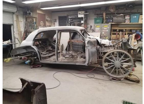
The wheels have been removed and now the long, daunting process of identifying the rear axle, all four hubs and spindles to order new bearings and brakes has started. We are awaiting estimates on sandblasting the wheels to determine the next step with them.
